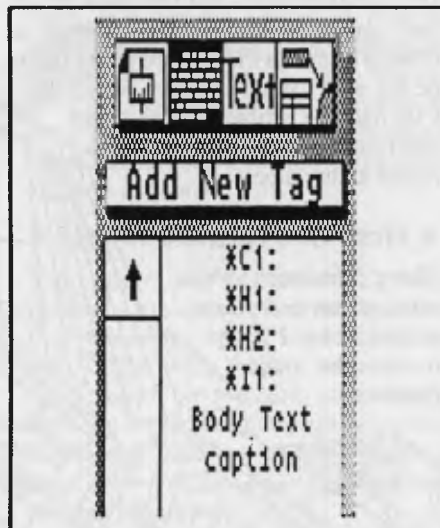
Above: This is a 'snapshot' of the Ventura side-bar menu. The four icons at the top represent the four modes - Frame, Tagging, Text editing and Drawing. We've selected Tagging, which brings up a list of tags associated with this document. This snapshot was taken from a standard IBM CGA screen.
